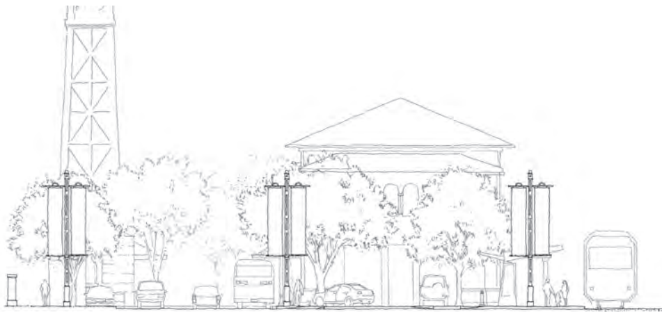
Top: Elevation view along Aurora Street showing steel entry archway and decorative fence and masonry piers; Above: Elevation along Weber Avenue showing steel entry piers supporting decorative banners.
