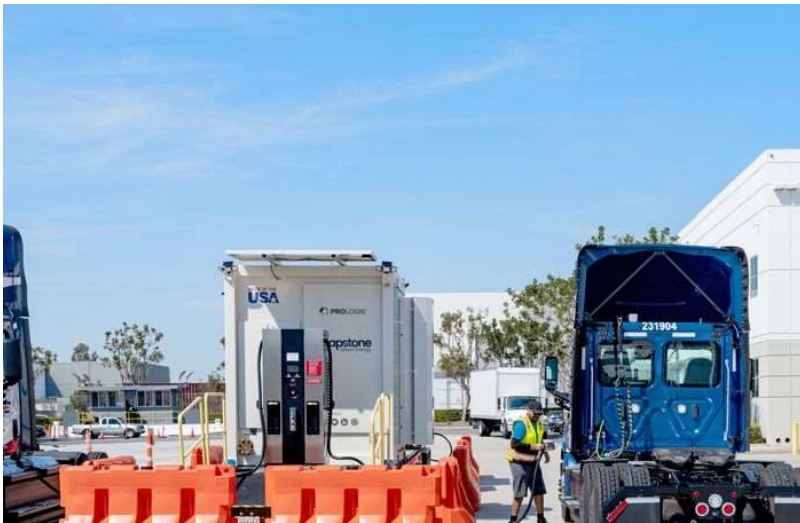
A mobile charging system in California runs on natural gas. PHOTO: PROLOGIS MOBILITY
