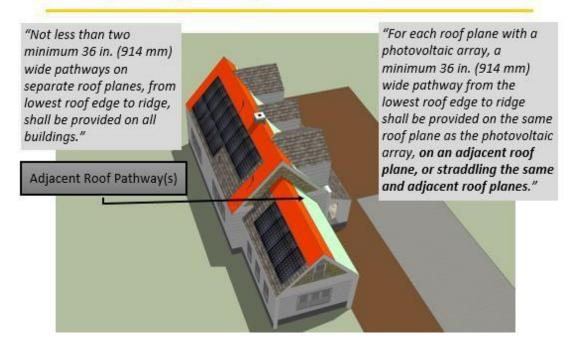
**R324.6.2 Setback at ridge.** For photovoltaic arrays occupying not more than 33 percent of the plan view total roof area, not less than an 18-inch (457 mm) clear set back is required on both sides of a horizontal ridge. For photovoltaic arrays occupying more than 33 percent of the plan view total roof area, not less than a 36-inch (914 mm) clear set back is required on both sides of a horizontal ridge.
