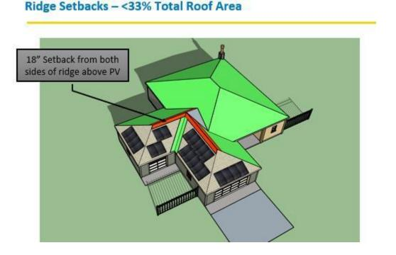
**R324.6.2.1 Alternative setback at ridge.** Where an automatic sprinkler system is installed within the dwelling in accordance with NFPA 13D setbacks at ridges shall conform with one of the following:
