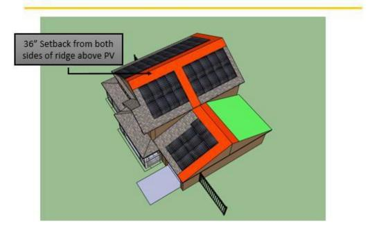
**R324.6.4 Emergency escape and rescue opening.** Panels and modules installed on dwellings shall not be placed on the portion of a roof that is below an emergency escape and rescue opening. A 36-inch-wide (914 mm) pathway shall be provided to the emergency escape and rescue opening.
